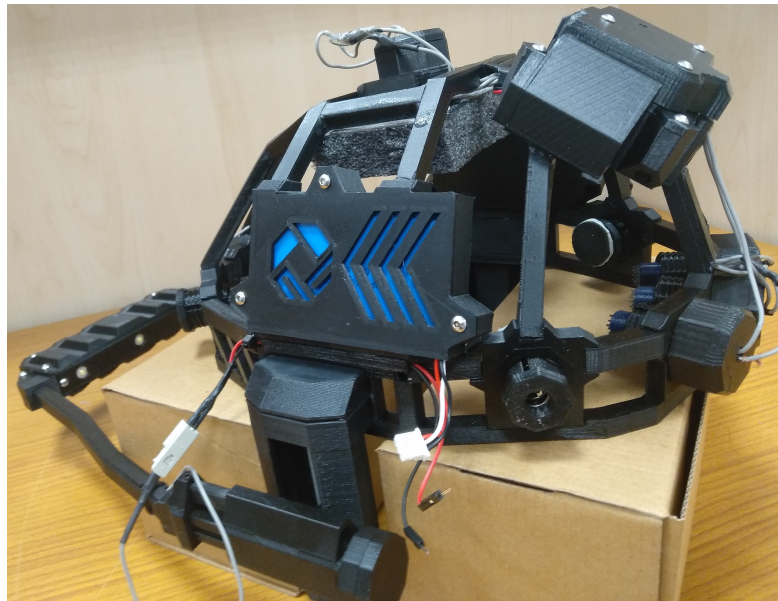
Figure 2.30: The complete 3D printed headset mounting 2 DC batteries, EEG data acquisition hardware, dry active electrodes, and the stimulator
