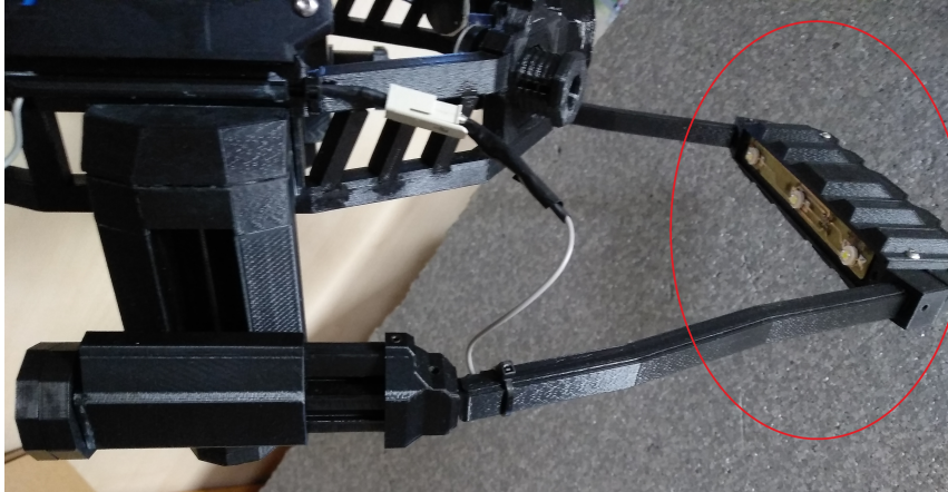
Figure 2.29: The stimulator part of the 3D printed headset (encircled) containing LEDs array and the stimulator circuit PCB
