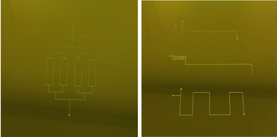
(a) Photomask for 8-branched microchannels. (b) Photomask with single channels, different geometries.
