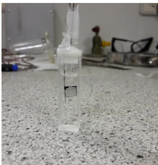
Figure 5. 13 The three electrode setup in a quartz cuvette.
