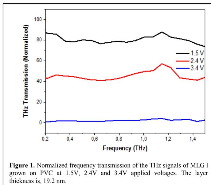
**Figure 1.** Normalized frequency transmission of the THz signals of MLG 1 grown on PVC at 1.5V, 2.4V and 3.4V applied voltages. The layer thickness is, 19.2 nm.
