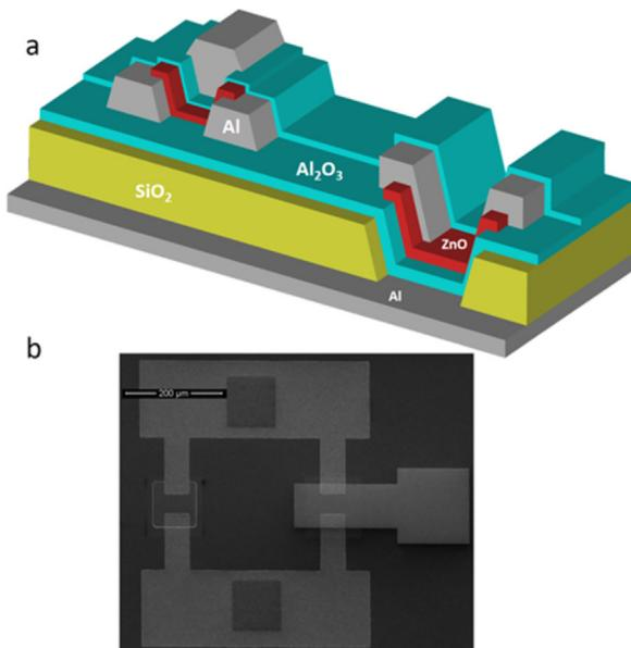
**Figure 1.** (a) 3D schematic of the vertically integrated TFTs. (b) SEM image of the fabricated devices.
