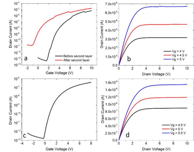
**Figure 2.** Electrical properties of TFTs on silicon substrates (a) bottom layer transfer characteristics. (b) Bottom layer output characteristics. (c) Top layer transfer characteristics. (d) Top layer output characteristics.
