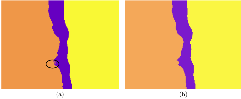
Figure 3.12: Illustration of the post-processing step on a sample image: (a) Resulting regions after the remapping operation. The circled area includes small regions that are byproducts of the remapping procedure. (b) Resulting segmentation after the extra small regions are eliminated by clean-up.
