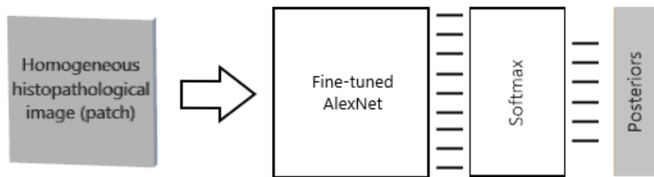
Figure 3.1: The end product of Tier 1. The desired CNN model after fine-tuning is expected to produce six posteriors that fairly characterize a homogeneous histopathological image. The decision layer indicated by “Softmax” is trained from scratch, to work as a classifier on top of the transferred information from previous layers of fine-tuned AlexNet. Details are specified in Section 3.1.1.
