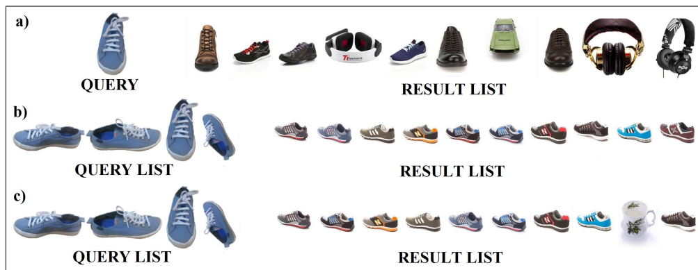
Figure 5.17: The results of single-view query object shoe (a), and Max (b), and Weighted Average Max methods (c), using multi-view database images
