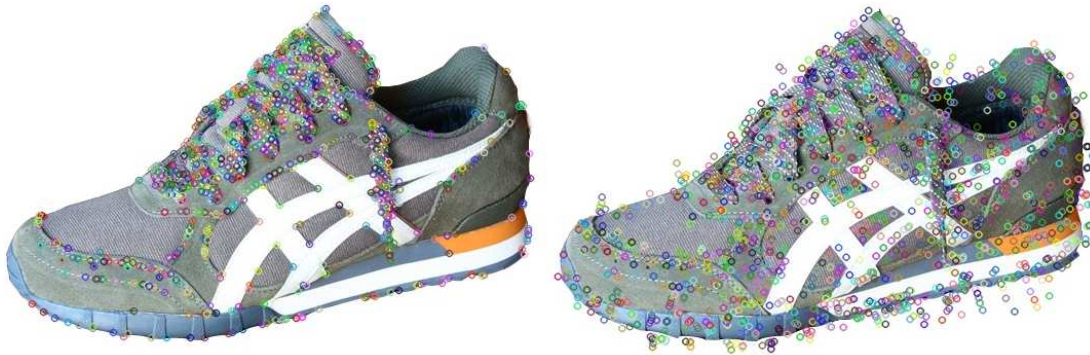
Figure 3.2: HARRIS (left) and SURF (right) key points detected in a query image
