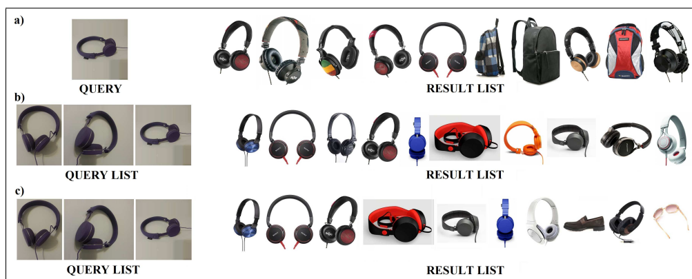
Figure 5.18: The results of single-view query object headphone (a), and Max (b), and Weighted Average Max methods (c), using multi-view database images
