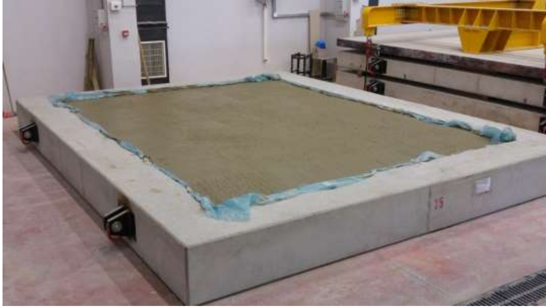
Figure 10. General view after concrete applied and finished sample slab without screed layer. (by Erdemli)
