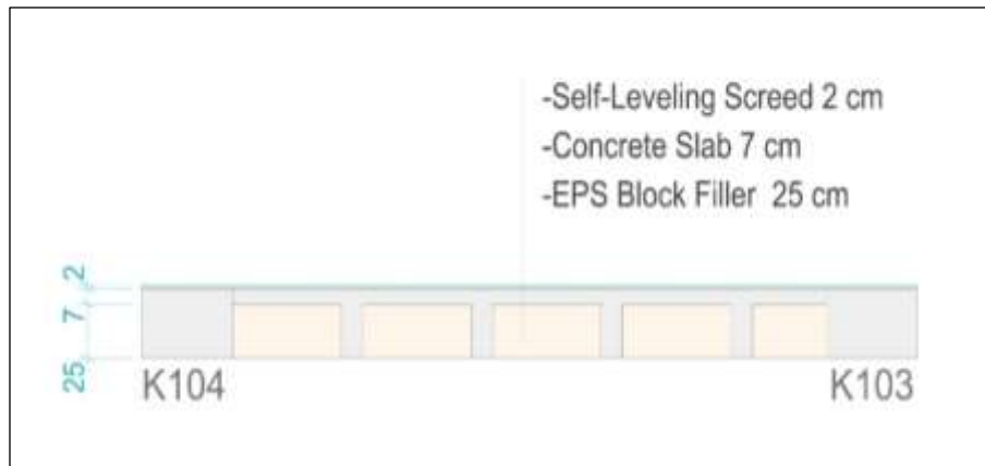
Figure 6. Section B of the sample one way hollow core slab system, not in scale (by Erdemli)
