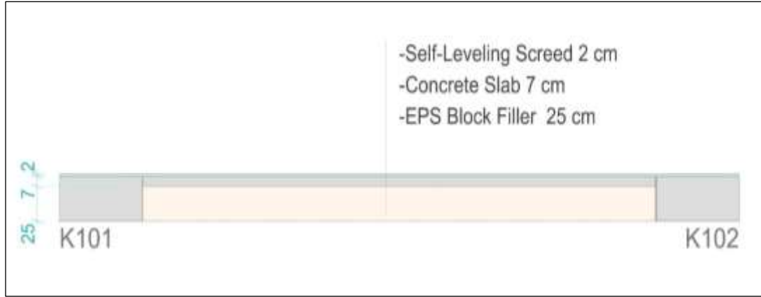
Figure 5. Section A of the sample one way hollow core slab system, not in scale (by Erdemli)
