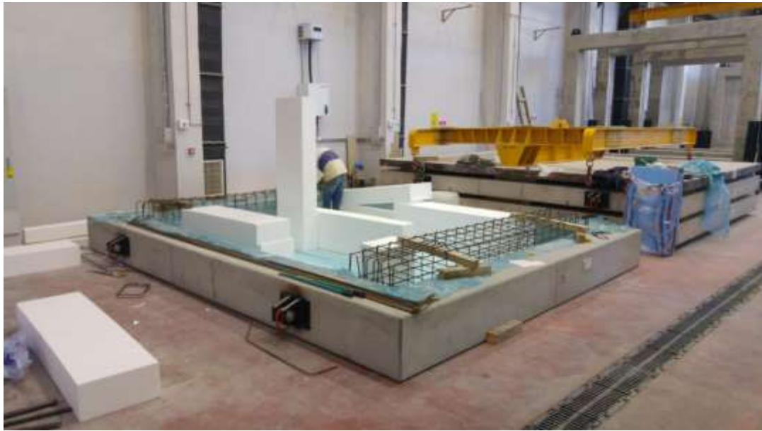
Figure 7. Reinforced concrete test frame and construction period (by Erdemli)
