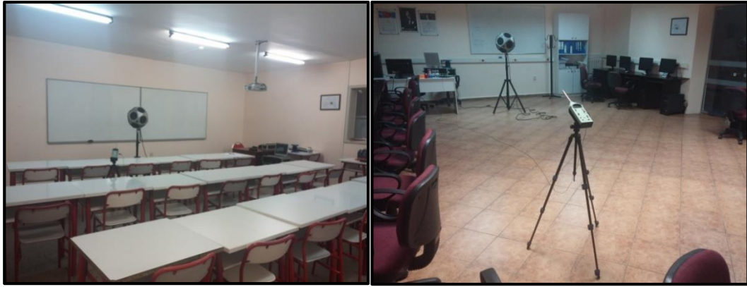
Figure 16: Measurement of reverberation time (T30) in classroom and computer laboratory environment
