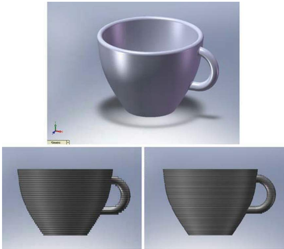
Figure 1.1: CAD image of a teacup with further images showing the effects of building using different layer thicknesses [1].
