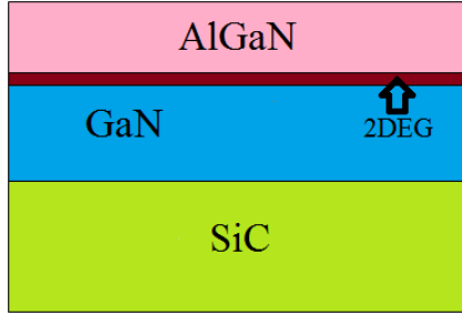
Figure 3.9: General HEMT device structure from side view
