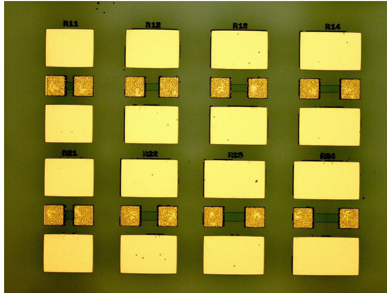
Figure 5.2: Fabricated Mesa resistors
