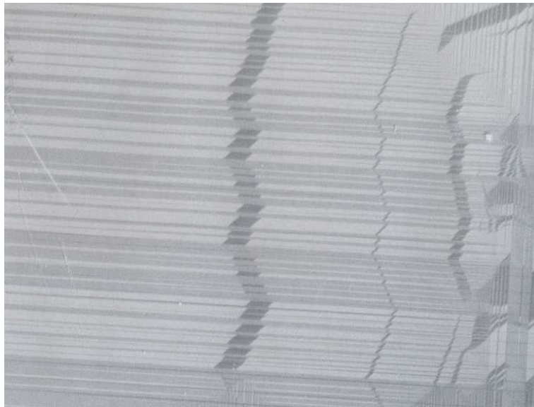
Figure 1.4: 50X magnification photo of LaAlO_3 . The twinning in LaAlO_3 is seen. (Photo by Rizwan Akram.)
