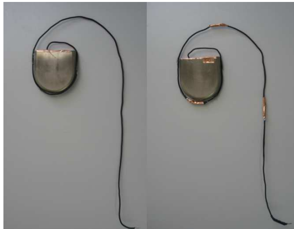
Figure 3.7: Home-made pacemakers. Left: The pacemaker that was modelled in the simulation. Right: Safe pacemaker in which RF chokes are placed with short intervals.
