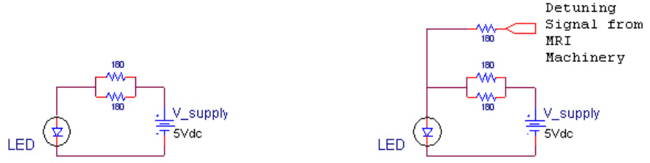
(a) Simple External Control Circuitry (b) Switching External Control Circuitry
