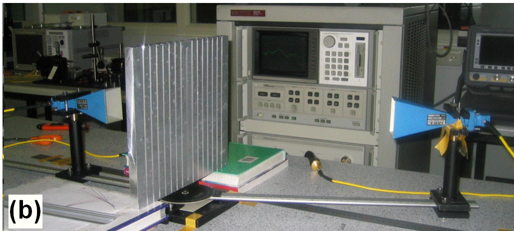
Fig. 4.1: (a) Schematic diagram of the transmission measurement setup. The setup consists of the network analyzer, two horn antennas and rotating arms. (b) Photograph of the transmission measurement setup.
