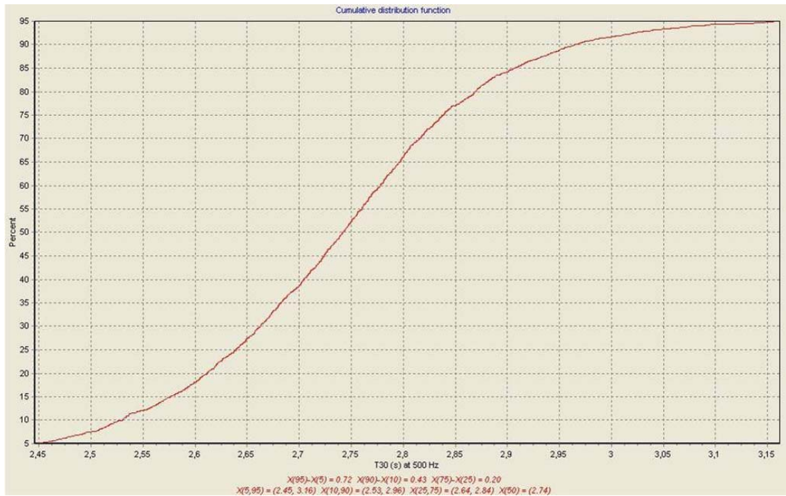
Figure 96. Reverberation time distribution graph for 500 Hz and for the renovated hall.
