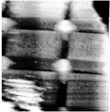
Figure 3.5: STM-tip image of a 4 \times 4 \mu\text{m}^2 GaAs grating, Loop Gain: 999, Vertical Range: 3 \mu\text{m} , Scan speed: 3 \mu\text{m/s} , Tunneling Current: -0.32 \text{ nA} , Bias voltage: -0.1 \text{ V}
