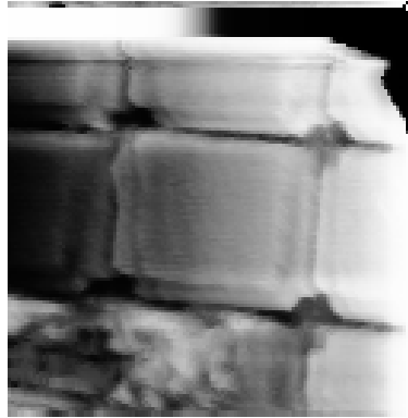
Figure 3.9: STM-tip image of a 4 \times 4 \mu\text{m}^2 GaAs grating, Loop Gain: 999, Vertical Range: 2.72 \mu\text{m} , Scan speed: 1 \mu\text{m}/\text{s} , Tunneling Current: -0.4 \text{ nA} , Bias voltage: -0.1 \text{ V}
