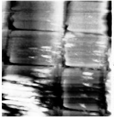
Figure 3.3: STM-tip image of a 4 \times 4 \mu\text{m}^2 GaAs grating, Loop Gain: 999, Vertical Range: 3.01 \mu\text{m} , Scan speed: 2 \mu\text{m}/\text{s} , Tunnelling Current: -0.35 \text{ nA} , Bias voltage: -0.1 \text{ V}
