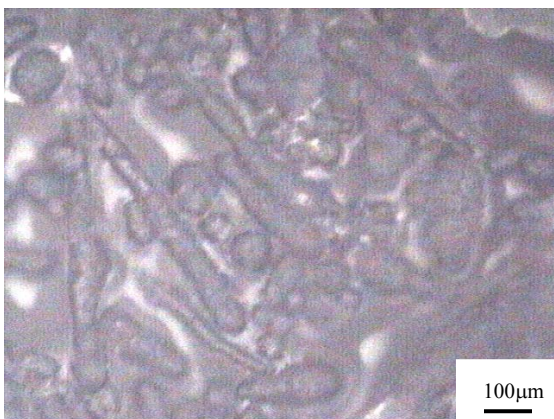
Figure 4.6: Optical micrograph of particles prepared in presence of 12.5 wt. % DVB (Experiment no. 11 in tables 3.1 and 4.1). (Magnification 100x).
