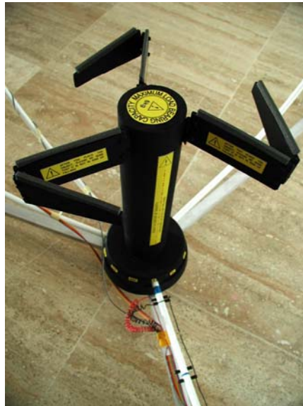
Figure 5.3. Adjustable base and object holding clamps.
