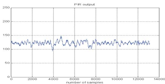
**Fig. 2.** A typical background PIR sensor output signal sampled at 100 Hz with 8 bit quantization when there is 'no activity' in its viewing range.
