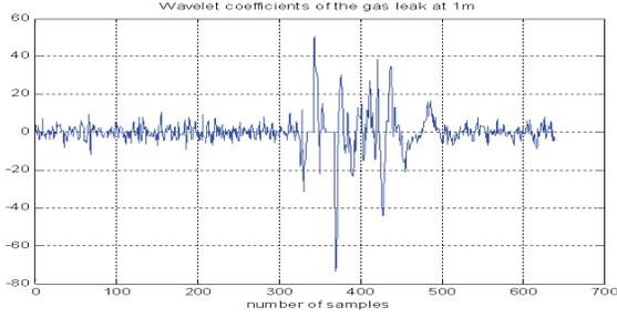
**Fig. 4.** Wavelet coefficients of the PIR sensor output signal recorded at a distance of 1m for the VOC gas leak shown in Figure 3(b).
