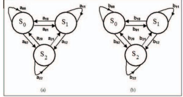
**Fig. 5.** Markov models and state transition definitions for (a) 'VOC gas leak' and (b) 'walking person' classes.
