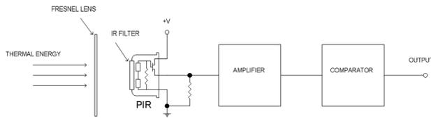
**Fig. 1.** The circuit diagram for capturing an analog signal output from a PIR sensor.
