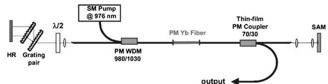
Fig. 1. Experimental setup of the mode-locked fiber laser.
