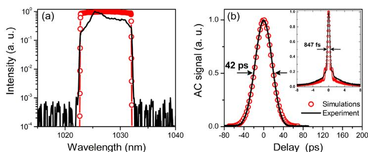
Fig. 2 : Output of the laser : typical output spectrum (a) and (b) output pulse autocorrelation. Inset : dechirped pulse autocorrelation.
