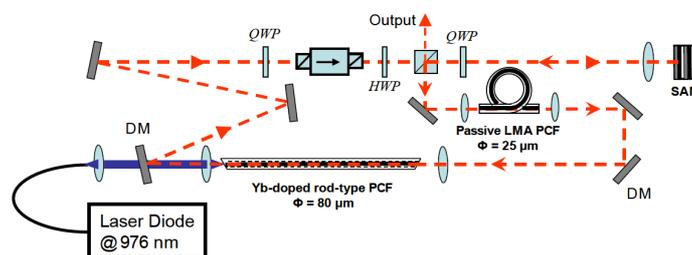
Fig. 1: Experimental setup of the chirped-pulse fiber oscillator
