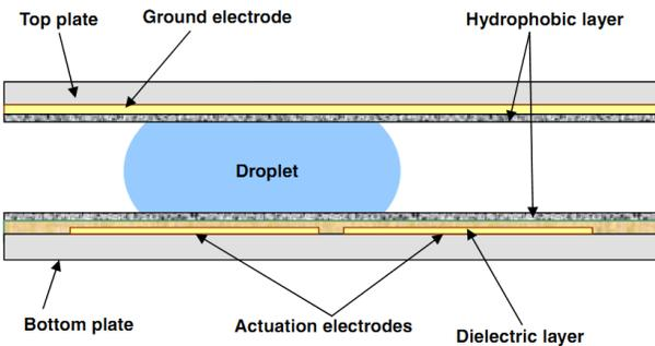
Figure 2: (a) An open setup EWOD device consisting of a metal electrode, the droplet to be actuated and a dielectric layer in between. (b) A closed setup EWOD device [7, 8]
