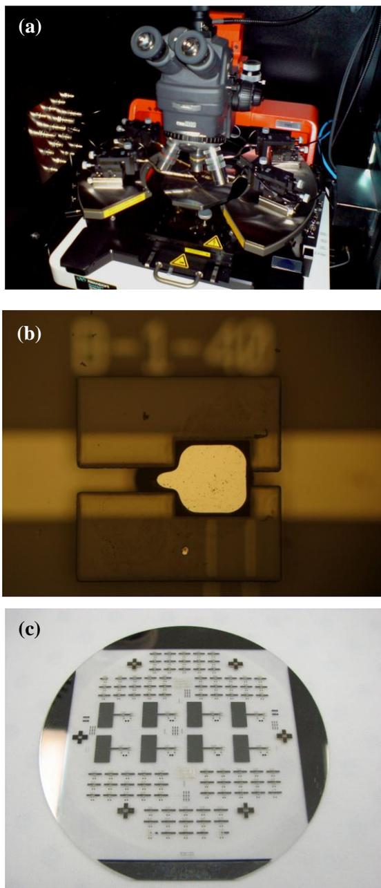
Figure 5: (a) The experimental setup used in this work: a probe station connected to a parameter analyzer; (b) A test device with a positioned metallic droplet; (c) a fabricated 4-inch quartz wafer with many test devices.
