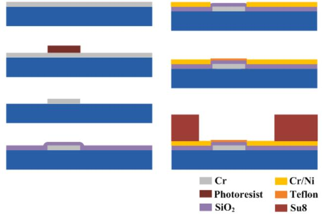
Figure 3: Micro-fabrication steps of test devices.
