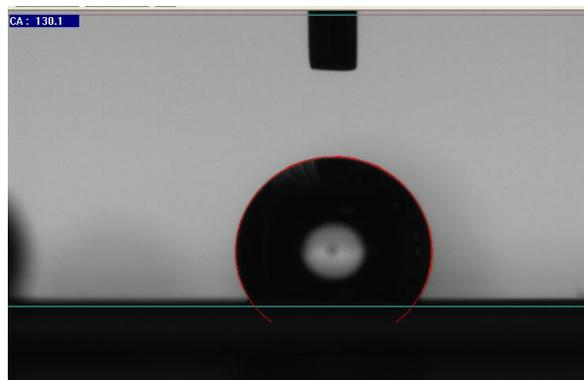
Figure 6: Contact-angle measurement of Teflon-coated surface
