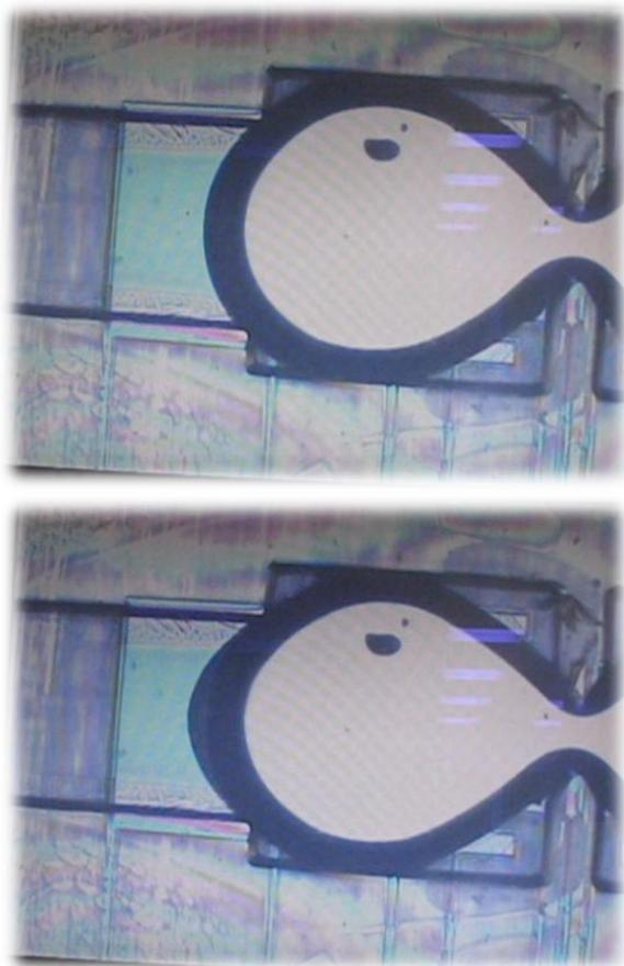
Figure 7: Top: Test device before actuation; Bottom: Actuation of the droplet with an actuation voltage of 100V.
