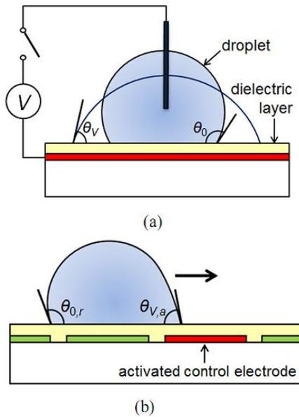
Figure 1: (a) EWOD device consisting of a metal electrode, the droplet to be actuated and a dielectric layer in between. (b) Actuation of a droplet on a device with more than one electrode [6]
