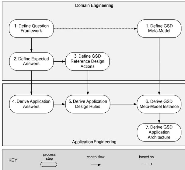
Figure 3. Process for deriving application architecture
