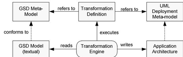
Figure 12. Model transformation pattern for mapping textual model to UML deployment view
