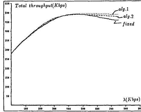
Figure 5: Total throughput versus internetwork load
