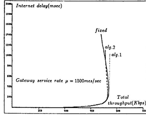
Figure 10: Average internet delay versus total throughput for different gateway service rates
