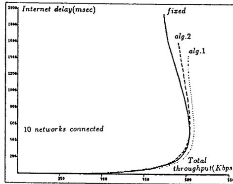
Figure 8: Average internet delay versus total throughput for different number of networks connected to internetwork
