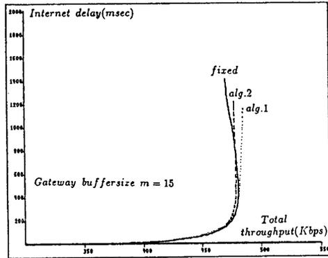
Figure 9: Average internet delay versus total throughput for different buffersizes of destination gateway
