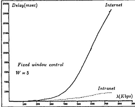
Figure 4: Average message delay versus internetwork load
