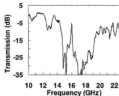
QThG6 Fig. 3. Normal  $0^\circ$  (100) incidence transmission through the MPC with the gap in the middle.
