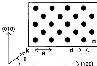
QThG6 Fig. 1. Top view of the (001)-oriented face of the MPC.
