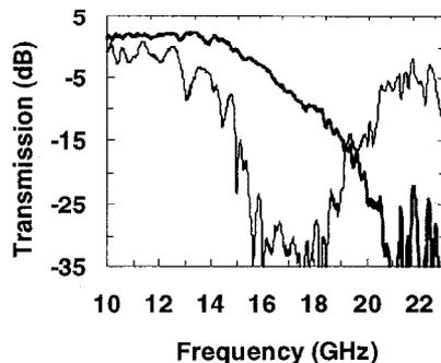
QThG6 Fig. 2. Normal  $0^\circ$  (100) (thin solid line) and  $45^\circ$  (110) (thick solid line) incidence transmission through the MPC.
