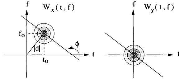
Figure 2: The non-central (left) and central (right) slices of the Wigner distribution  $W_x(t, f)$  and  $W_y(t, f)$ .
