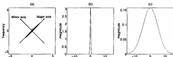
Figure 1: A chirp signal has a low-pass characteristic along its major axis (b), and it has considerable bandwidth in along its minor axis (c).
