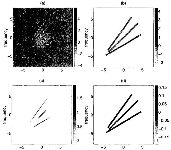
Figure 3: The Wigner distribution (a), slices of the Wigner distribution (b), slices of the Wigner distribution smoothed with data-adaptive directional filtering (c), the difference of the smoothed slices from the auto-components only.
