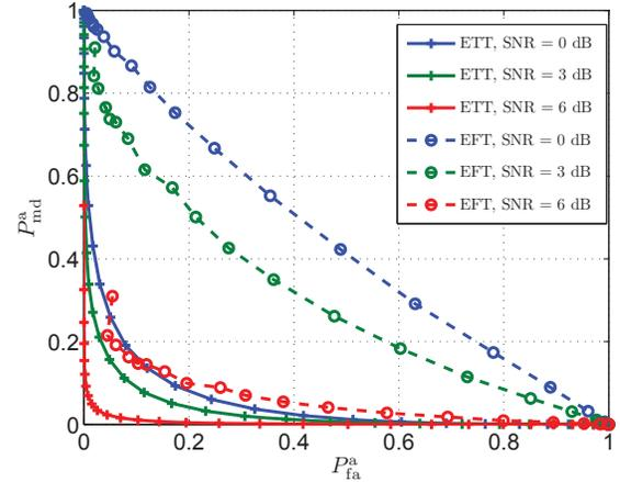
**Fig. 2:** Operating characteristic  $P_{md}^a$  vs  $P_{fa}^a$  for  $T = M$
