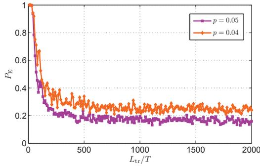
Fig. 3: Probability of wrong estimation  $P_E$  as a function of  $L$  for  $T = M$ , SNR = 5 dB
