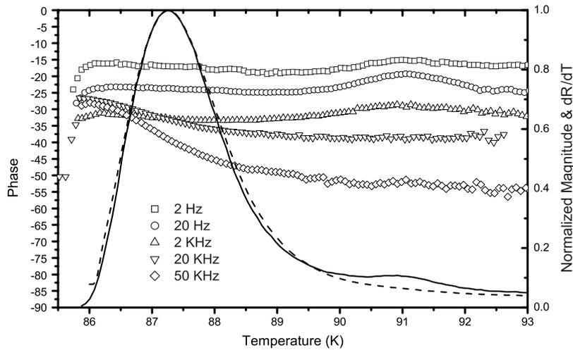
**Figure 1.** The temperature dependence of the phase (scatter plots) and magnitude (solid line) of the IR response and  $dR/dT$  (dash line) of large area bolometer on  $LaAlO_3$  substrate.
