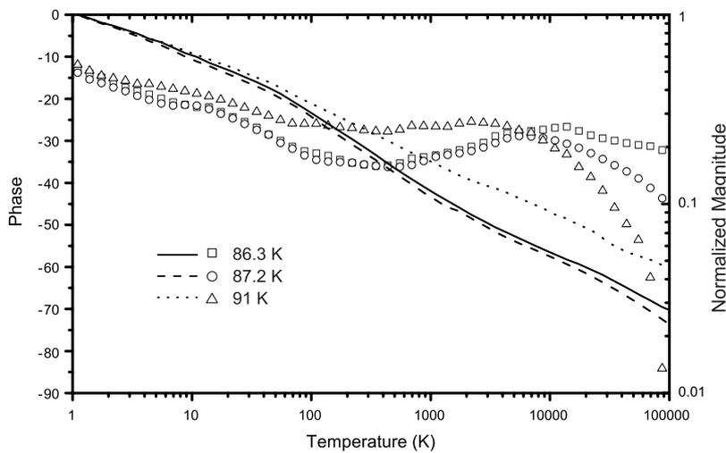
**Figure 2.** The phase (scatter plots) and magnitude (solid line) of the IR response versus frequency measured at temperatures  $T_{c-zero}$ ,  $T_c$  and  $T_{c-onset}$  for large area bolometer on  $LaAlO_3$ .
