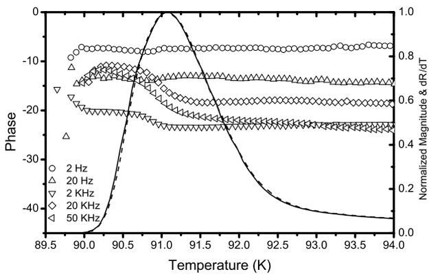
**Figure 4.** The temperature dependence of the phase (scatter plots) and magnitude (solid line) of the IR response and  $dR/dT$  (dashed line) of first type small area bolometer on LaAlO<sub>3</sub> substrate.
