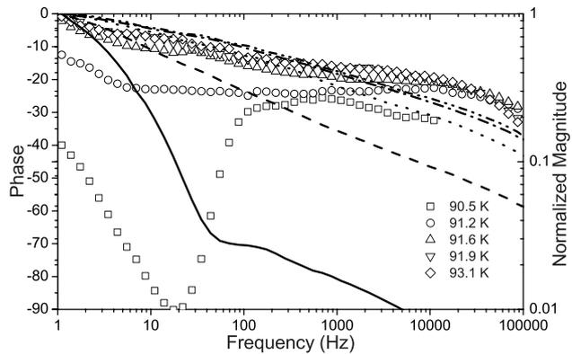
**Figure 6.** The phase (scatter plots) and the magnitude (solid line) of the IR response versus frequency measured at temperatures around  $T_c$ ,  $T_{c-zero}$  and  $T_{c-onset}$  for second type small area bolometer on LaAlO<sub>3</sub>.
