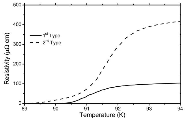
**Figure 7.** Resistivities of first and second type small area bolometers on LaAlO<sub>3</sub> substrate for demonstrating the correlation between the resistivity and the optical response of the devices. (See figures 5 and 6.)
