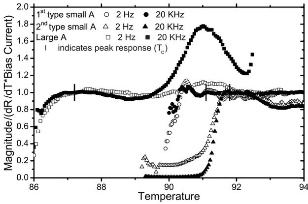
**Figure 3.** Magnitude of the response normalized with respect to the derivative of the resistance and the bias current for large area and small area bolometers on LaAlO<sub>3</sub>.
