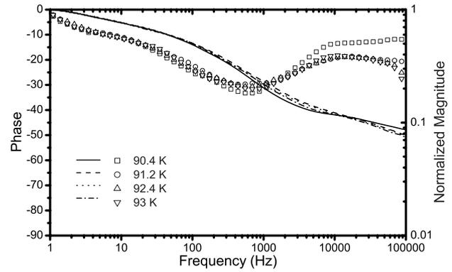
**Figure 5.** The phase (scatter plots) and the magnitude (solid line) of the IR response versus frequency measured at temperatures around  $T_c$ ,  $T_{c-zero}$  and  $T_{c-onset}$  for first type small area bolometer on LaAlO<sub>3</sub>.
