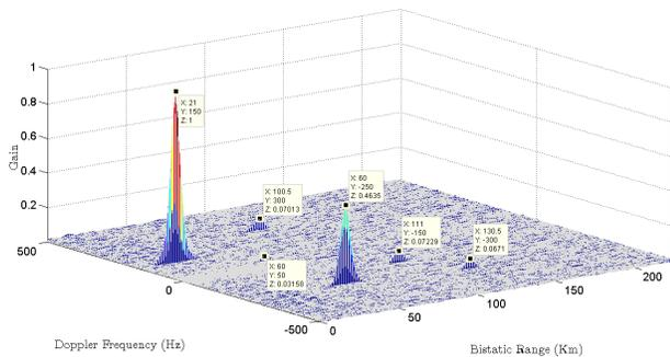
**Fig. 1:** 3-D range-Doppler frequency graph obtained using AF computed using FFT as in Equation 5.
