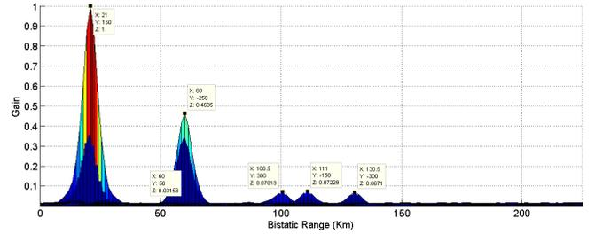
**Fig. 3:** Bistatic range graph obtained using AF computed using FFT as in Equation 5.
