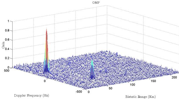
**Fig. 6:** Range-Doppler map for OMP algorithm.
