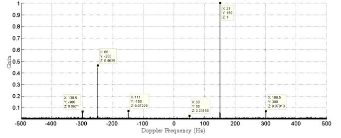
**Fig. 2:** Doppler frequency graph obtained using AF computed using FFT as in Equation 5.
