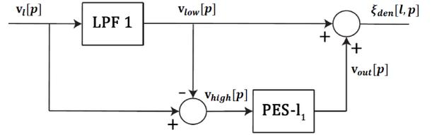
Fig. 4: The block diagram of PES- $\ell_1$  algorithm.
