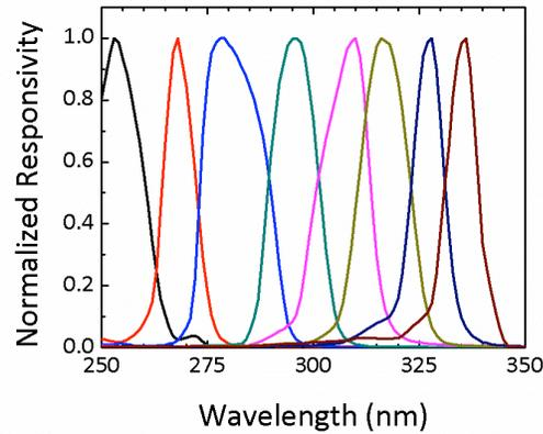
Fig. 4. Normalized responsivity of wavelength sensitive monolithic stack of MSM photodetectors.
