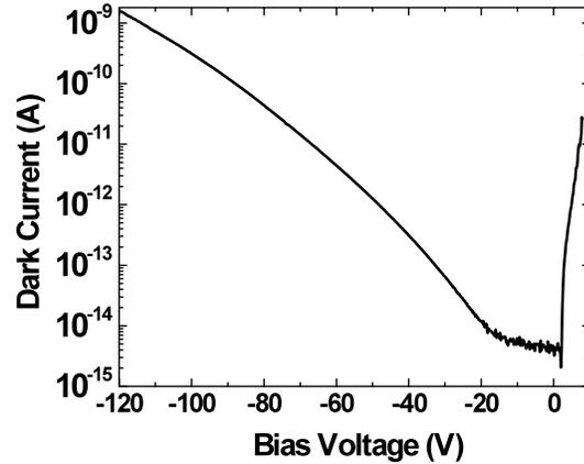
Fig. 2. Dark current of a 200 µm diameter AlGaIn p-i-n photodetector.
