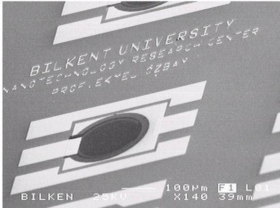
Fig. 1. SEM image of 200 micron diameter fabricated device
