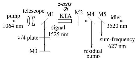
Fig. 1. Experimental setup of the SF-OPO.
