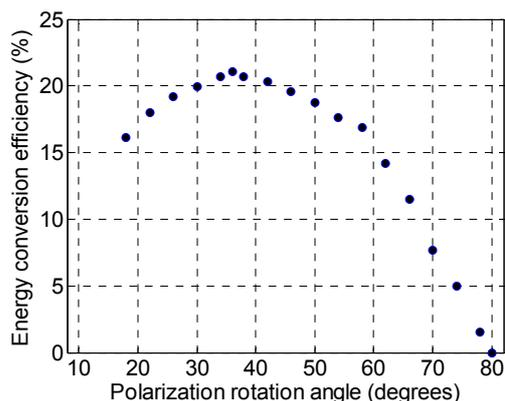
Fig. 2. Sum-frequency conversion efficiency as a function of the polarization rotation angle. Pump pulse energy is held fixed at 39.2 mJ.
