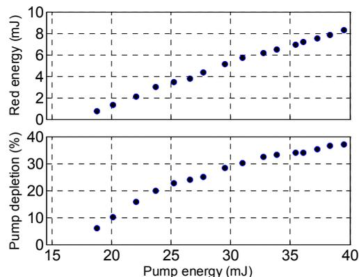
Fig. 3. Sum-frequency pulse energy and pump depletion as functions of pump pulse energy. Polarization rotation angle is held fixed at  $36^\circ$ .
