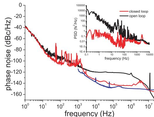
Figure 6: Single sideband phase noise of the Bates Master Oscillator (MO) (black), the EDFL locked to the reference after transmission through the link (red) and the free running EDFL (blue). Inset: Mixer output signal of the RF fiber link stabilization.
