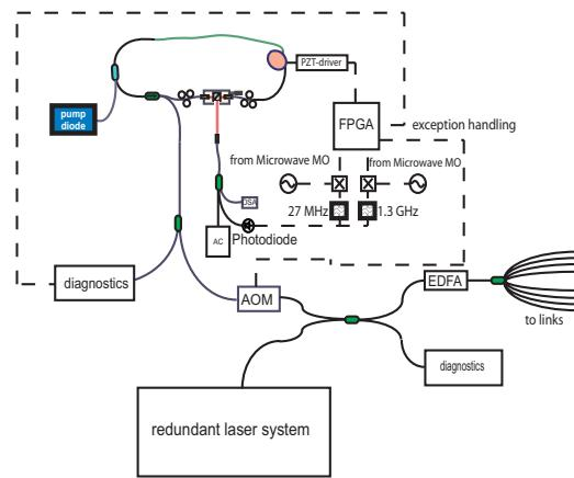
Figure 7: Schematic of the LMO System for the FEL facility FLASH at DESY
