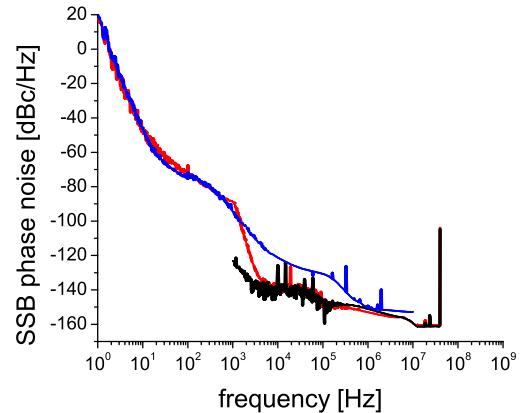
Figure 3: Spectral density of single-sideband phase noise for the free-running EDFL (black), the RF reference oscillator used to lock the EDFL (blue), and the EDFL locked to the reference (red).
