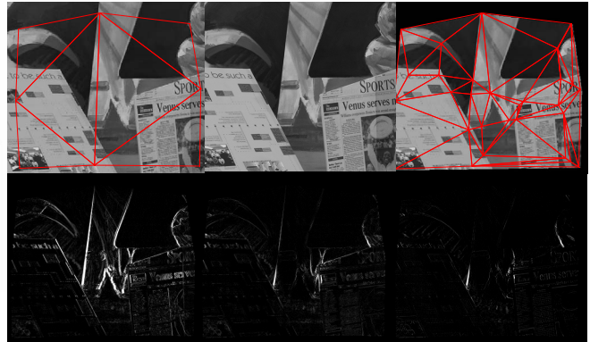
Figure 3: “Venus” Top row, left to right: Reference and target and predicted frames. Bottom row, left to right: Initial error, error before non-linear refinement, error after non-linear refinement. Errors are scaled by 3 to enhance visibility. Reference frame is overlaid with the projection of the initial mesh, and predicted frame, with the projection of the 30-vertex mesh
