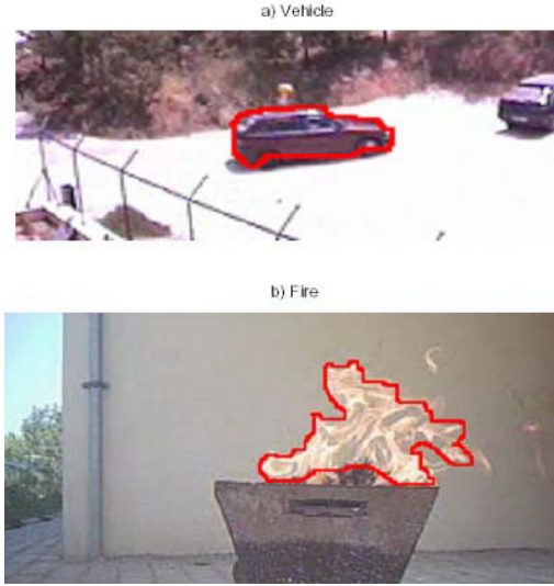
Figure 3. Two fire-colored moving objects in video: a) a vehicle, and b) fire image. Moving objects are determined by the hybrid background subtraction algorithm of [6].
