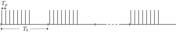
Fig. 1. Transmitted signal structure for estimation of vital signal parameters. Pulses in each burst are used to improve signal-to-noise ratio (SNR) at the receiver, and different bursts give information about vital parameters, such the respiration rate.
