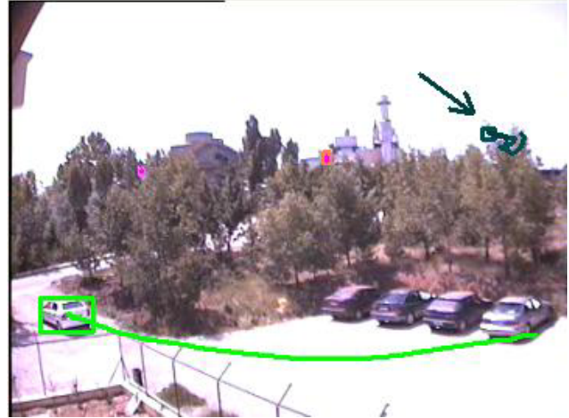
Fig. 2. The car has a directionally consistent trajectory whereas the leaves, pointed with an arrow, sway randomly in the wind
