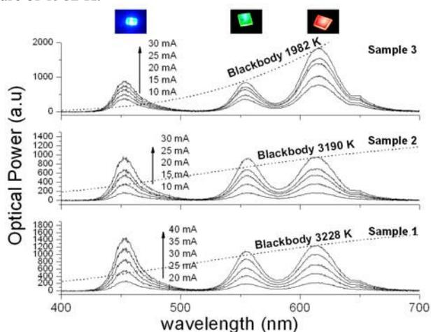
**Figure 2.** Luminescence spectra of our nanocrystal hybridized warm-white LEDs (Samples 1-3) when electrically driven at room temperature.
