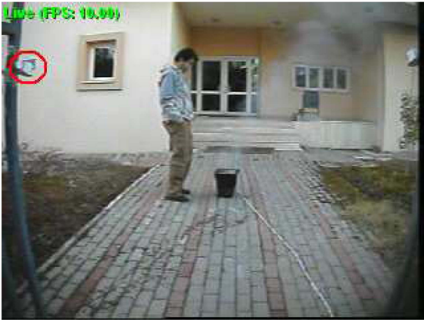
Figure 7: The PIR sensor is encircled. The fire is close to die out completely. A man is also within the viewing range of the sensor.
