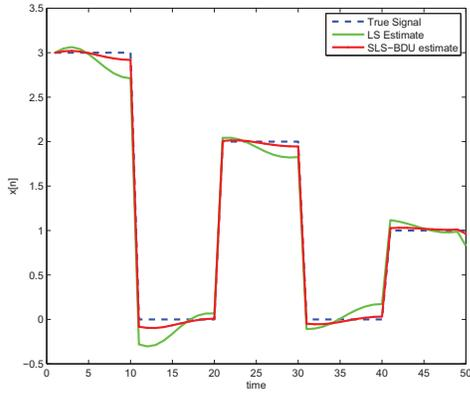
**Fig. 2.** Actual and restored signals are shown in dashed and solid lines respectively.
