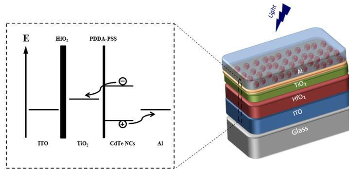
**Figure 1.** Schematic of the proposed LS-NS device with the energy band diagrams of CdTe NCs, TiO<sub>2</sub>, ITO and Al. When the excitons are photogenerated, electrons are transferred to the TiO<sub>2</sub> layer while holes migrate to the Al layer.
