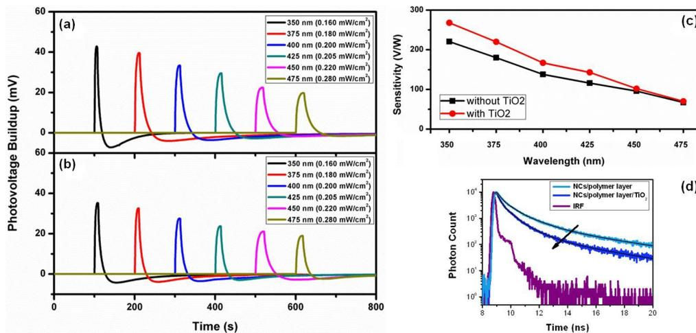
**Figure 2.** Photovoltage buildup at different excitation wavelengths for the LS-NS (a) with TiO<sub>2</sub> and (b) without TiO<sub>2</sub>. (c) Demonstration of device sensitivity enhancement at different excitation wavelengths and (d) time resolved fluorescence decay lifetime shortening of the LS-NS with and without TiO<sub>2</sub>.
