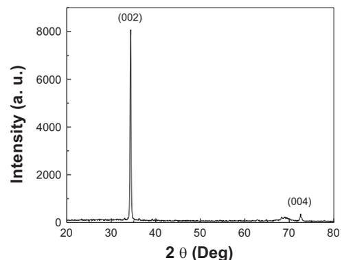
Fig. 3. XRD spectrum of ZnO:Ga/graphene thin film.
