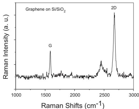
Fig. 5. Raman spectrum of graphene transferred onto SiO<sub>2</sub>/Si substrate.
