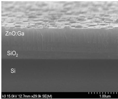
Fig. 4. SEM cross-section image of ZnO:Ga/graphene/SiO<sub>2</sub>/Si.
