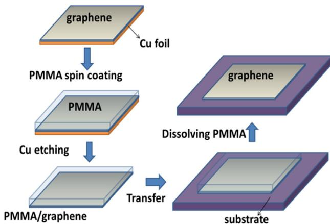
Fig. 1. Schematic diagram of graphene transfer onto substrate.
