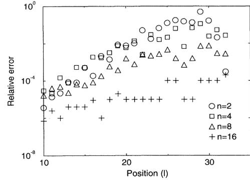
FIG. 2. The relative error in the wave function at  $t = 15$  of Fig. 1, displayed for various values of the size  $n$  of the boundary region. The relative error is defined as  $|\psi_l/\Psi_l - 1|$ , where  $\psi_l$  and  $\Psi_l$  are the values of the wave function on a simulation mesh of sizes 32 and 128, respectively.
