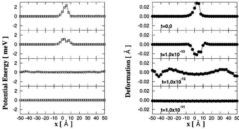
FIG. 2. Propagation of the local potential (strain) energy and deformation created in an infinite 1D substrate. Atoms are allowed to move in the  $x$  direction since  $k_z$  is taken to be infinite.
