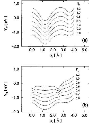
FIG. 4. Total potential  $V_T$  versus  $x_t$  calculated for various normal forces  $F_N$  in nN. (a) Rigid substrate in the perpendicular direction, i.e.,  $k_z=\infty$  and (b)  $k_z=10$  eV/Å<sup>2</sup>.
