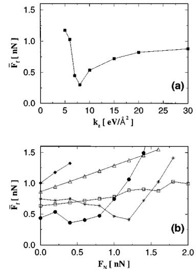
FIG. 5. (a) Variation of the average friction force as a function of force constant in the perpendicular direction  $k_z$ .  $F_N=0.2$  nN. (b) Average friction force versus normal loading force  $F_N$  calculated for various  $k_z$ . Filled squares, triangles, stars, filled circles, and empty squares correspond to  $k_z=5, \infty, 15, 10$  eV/Å<sup>2</sup>, and anharmonic  $V_{p,i}$ , respectively.
