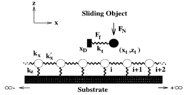
FIG. 1. Atomic model used to study the friction force  $F_f$  and the stick-slip motion.  $F_N$  is the normal loading force,  $(x_t, z_t)$  are the coordinates of the moving agent represented by a single atom,  $x_D$  is the position of the moving agent, and  $k_t$ ,  $k_x$ ,  $k_x'$ , and  $k_z$  are the spring constants described in the text.
