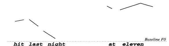
Fig. 4. Schematic example of stylized F0 for voiced regions of the text. The speaker’s estimated baseline F0 (from the log-normal tied mixture modeling) is also indicated.
