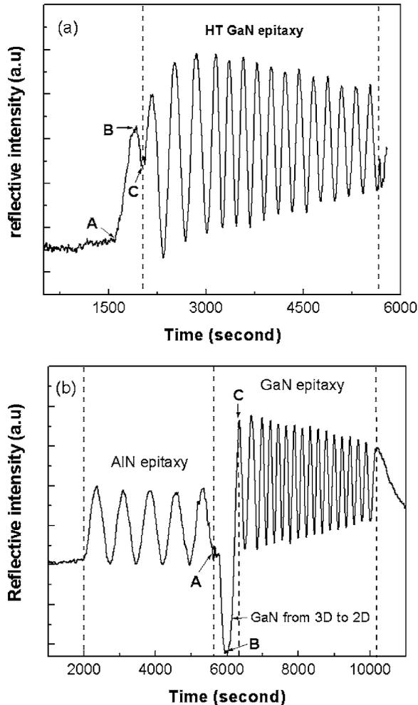
FIG. 4. Reflectivity monitored during semi-insulating GaN epitaxy on (a) LT-GaN nucleation and (b) AIN buffer. The 3D-2D transition is clearly visible in GaN grown on AIN buffer.
