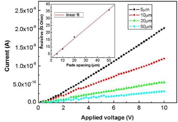
FIG. 2. (Color online) Dark  $I$ - $V$  characteristics of sample A obtained from a set of TLM pads.
