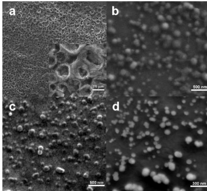
Fig. 2. SEM micrographs of films prepared from (a) PF solution, (b) PF NP dispersion (c) MEH-PPV $\mathbf{a}$  NP dispersion, and (d) (MEH-PPV $\mathbf{a}$ /PF) sequential NP dispersion. The last image is taken with a tilt angle of 15°.
