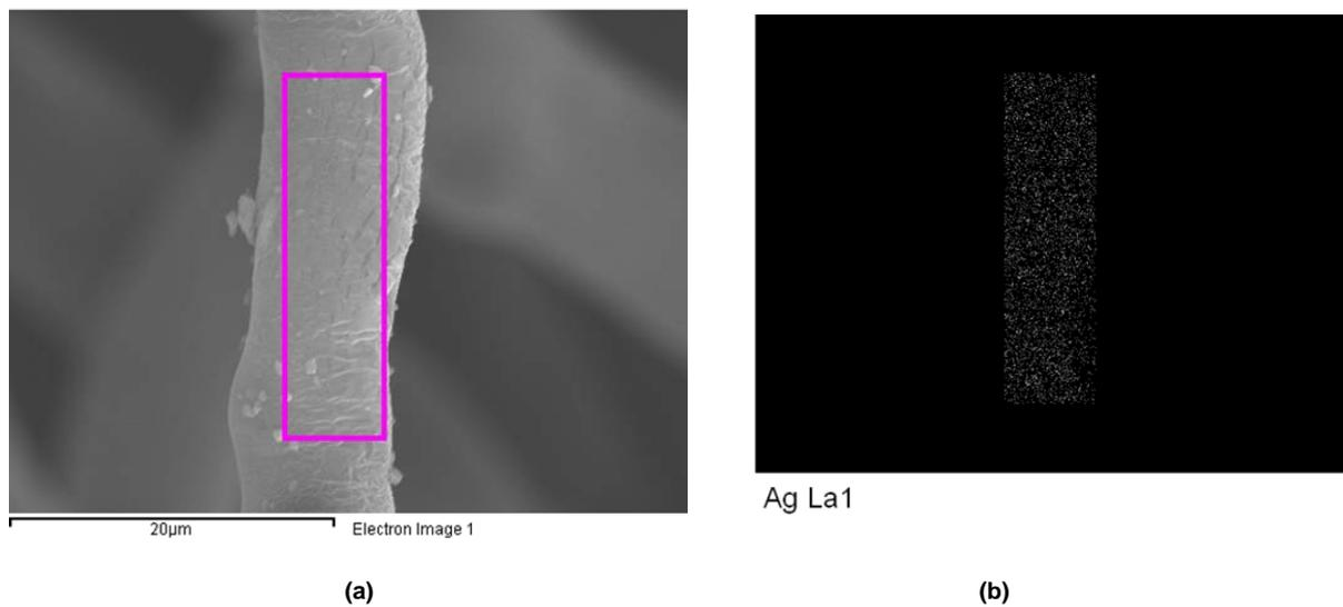
**Figure 3.** a) SEM image of the SCA fiber; b) EDX mapping result of Ag La1 corresponding to selected area of (a) (SEM accelerating voltage = 20 kV)
