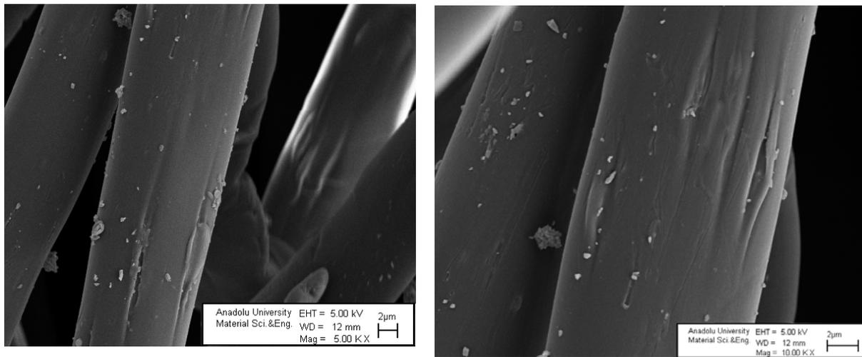
**Figure 2.** SEM images of SeaCell Active fibers (magnified 5,000 and 10,000 times)
