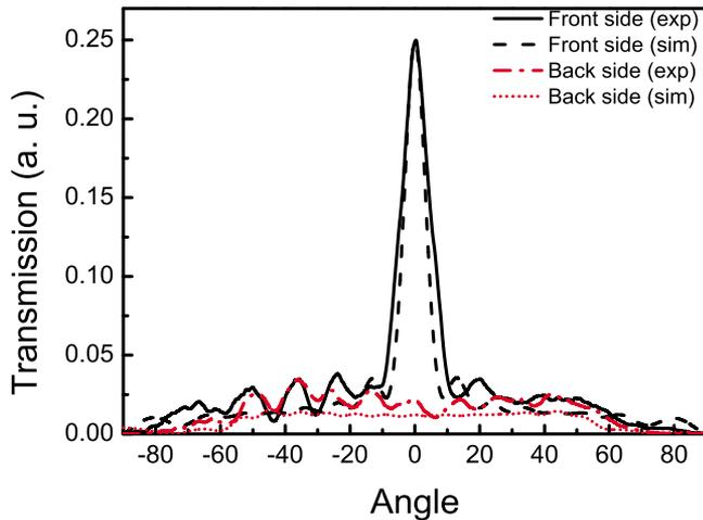
FIG. 4. (Color online) Experimental and simulated angular distributions of transmission at  $f=9.8$  GHz for sample A at  $\theta=30^\circ$ . Positive angles represent the right-hand side of the structure, while negative angles represent the left-hand side of the structure.
